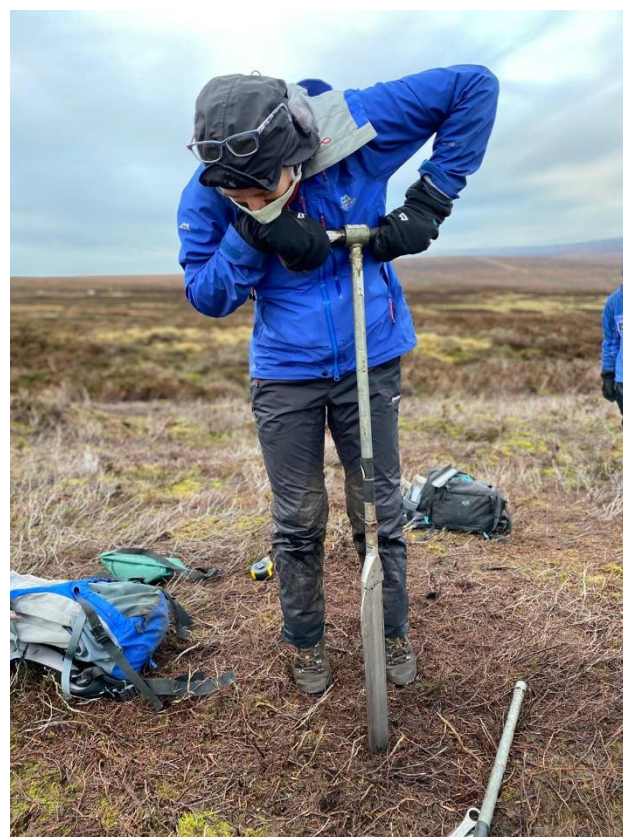
Figure 5-2: Using a Russian corer to retrieve a peat core from 30 cm to full peat depth (image by John Moore, University of Manchester)
