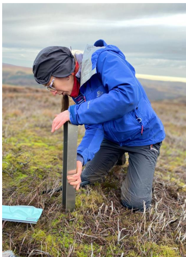
Figure 5-1: Using a box corer to retrieve a peat core from the surface to a depth of 50 cm (image by John Moore, University of Manchester)
