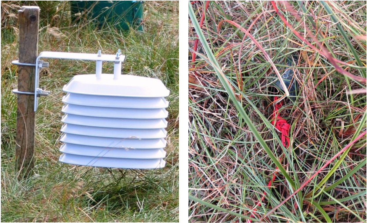
Figure 41. Air temperature logger within solar radiation shield (left) and soil temperature logger (right).
