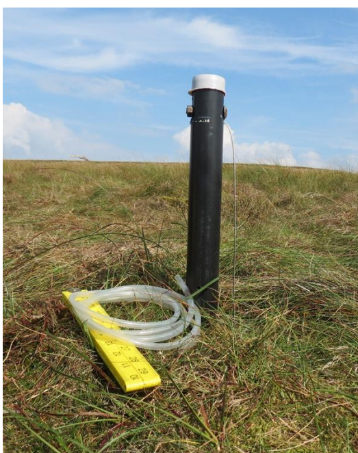
Figure 48. Automatic water table depth logger (left) and measurement being taken from a manual dipwell (right).
