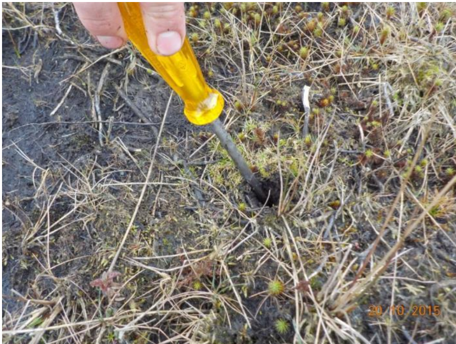
Figure 43: Make a hole deep and wide enough to fit in the plug
