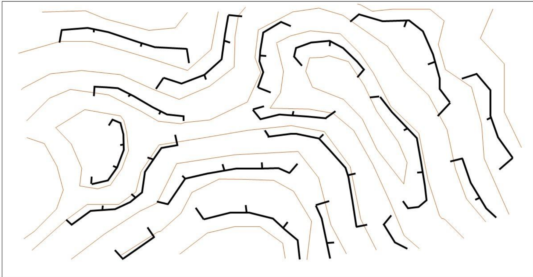
Figure 46: Illustrative contour trench bund arrangement
