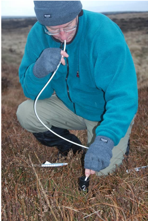
Figure 6.3: Surveyor measuring water level within a manual dipwell
