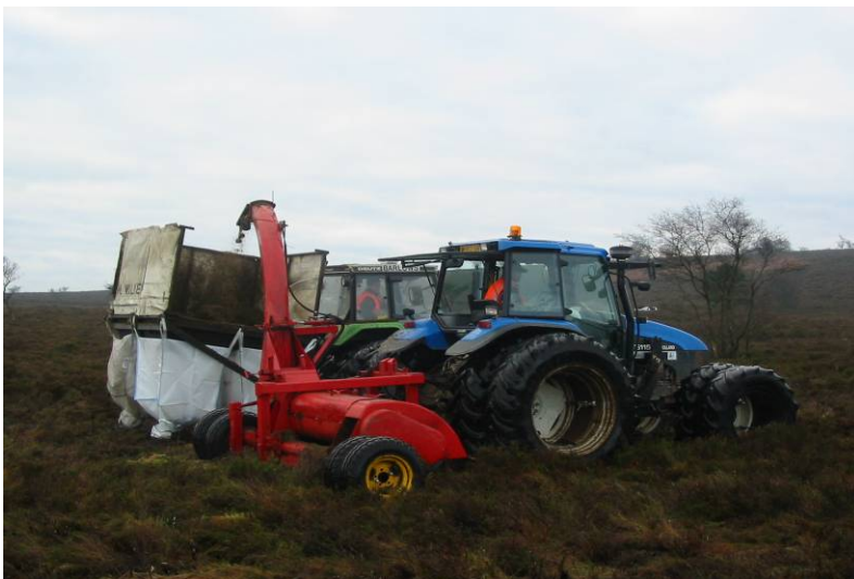
Figure 1. Heather brash cutting on Warslow Moors using a double chop forage harvester
