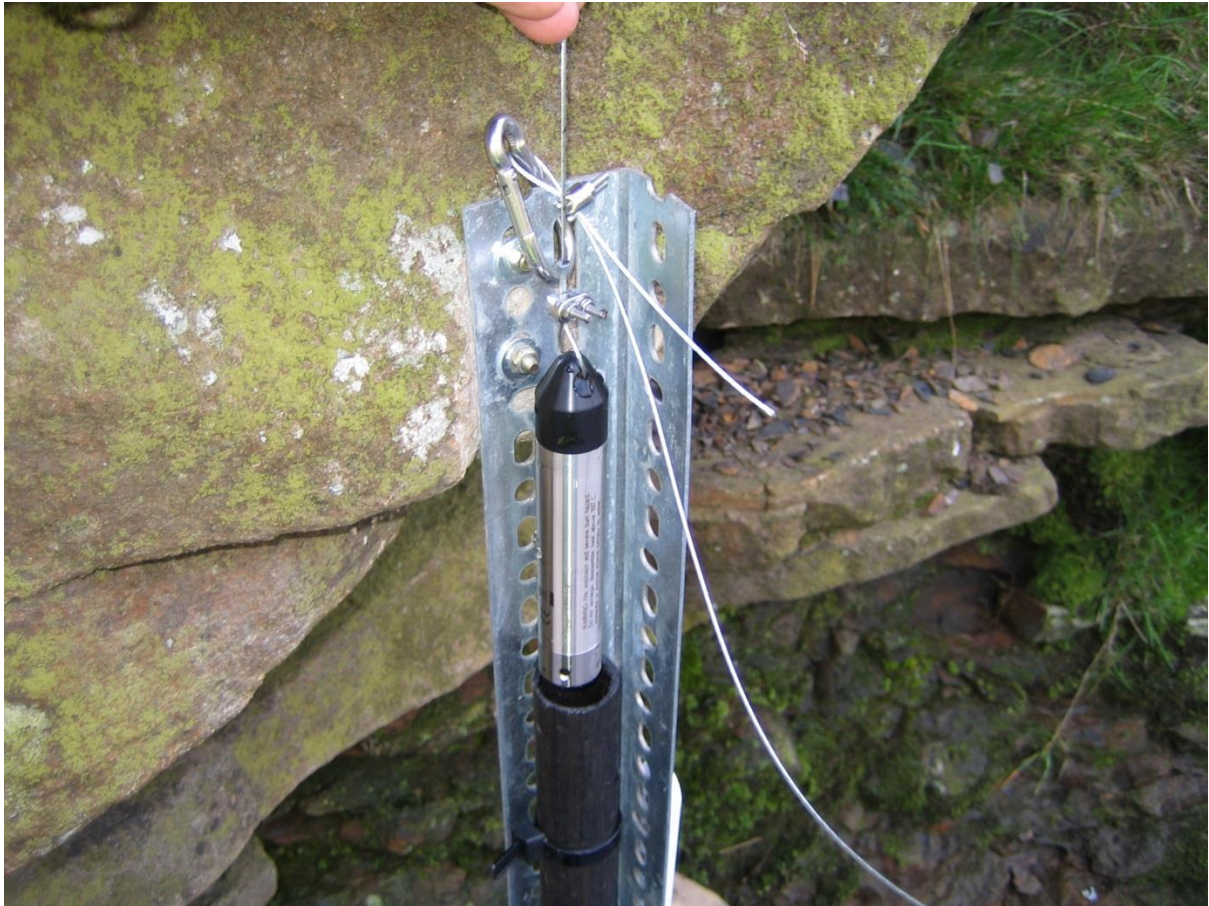
Figure 7.8: HOBOT water level data logger suspended inside plastic pipe
