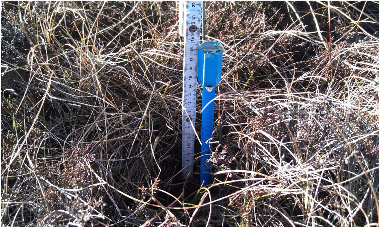
Figure 7.3: A peat anchor at Oyster Clough
