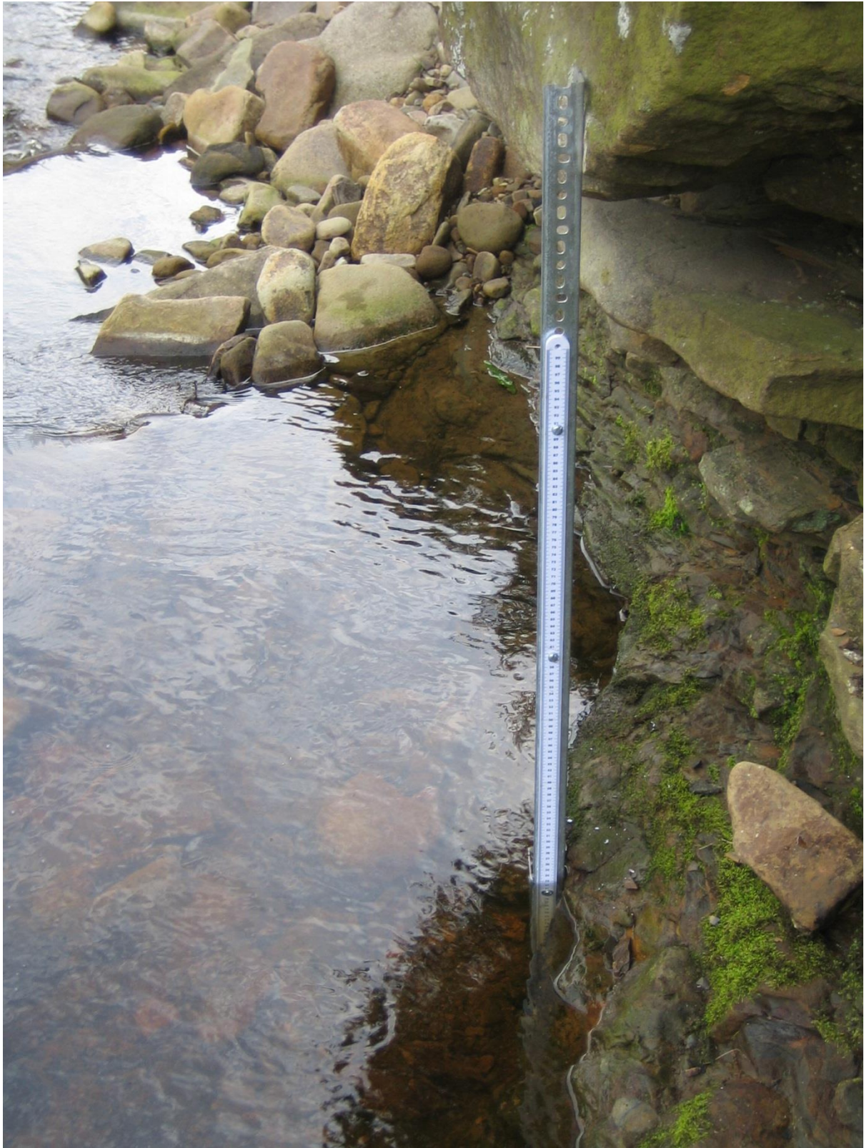
Figure 7.6: Dexion structure and ruler for measuring stage height
