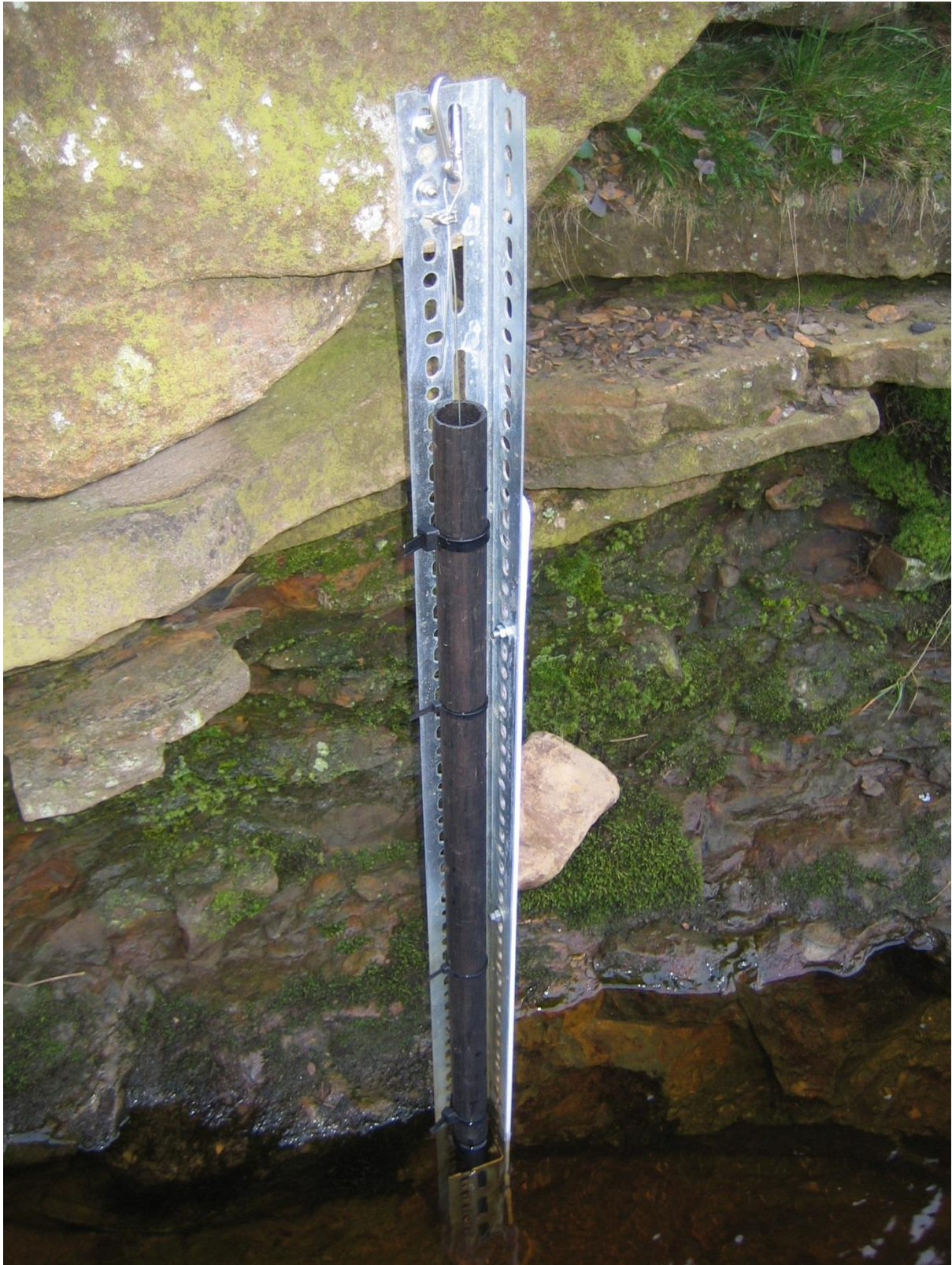
Figure 7.7: Plastic pipe attached to dexion structure
