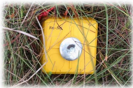
Figure 33: Newly installed automatic water table loggers (left), rainfall gauges, humidity loggers and surface temperature loggers can all be easily downloaded with small, lightweight shuttles (right) then viewed by volunteers at home using software supplied.
