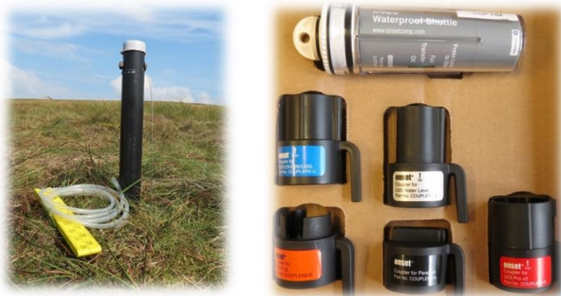
Figure 33: Newly installed automatic water table loggers (left), rainfall gauges, humidity loggers and surface temperature loggers can all be easily downloaded with small, lightweight shuttles (right) then viewed by volunteers at home using software supplied.
