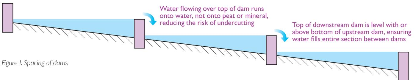
Figure 1: Spacing of dams
